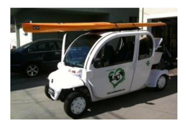
**Description:** The GEM e4 is a compact 2-door (butterfly style) all electric vehicle. It seats four people with a rear external trunk box. Aside from windshield wipers and seatbelts the GEM e4 does not feature any other amenities.
