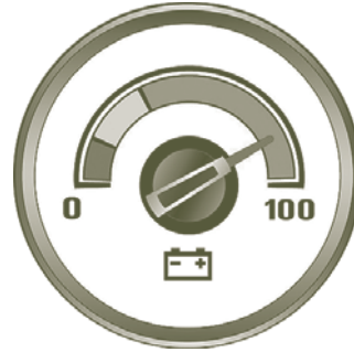
Battery Discharge Indicator
